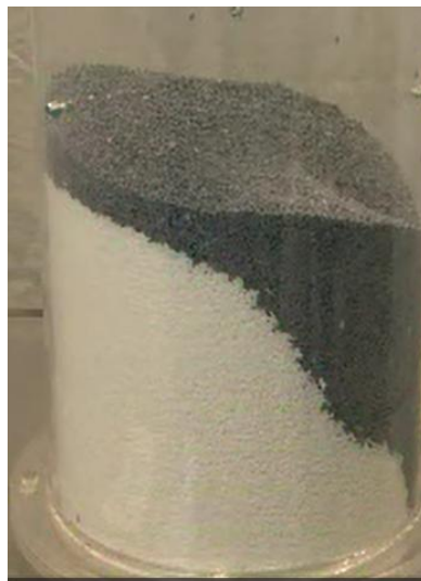
Figure 28: Gravity dumping of free flowing catalyst LIFO Pattern
