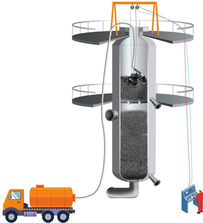
Figure 21: Caterpillar vacuum device scrawling at the surface of the catalyst
