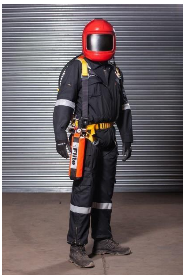
Figure 5: Example of life support system (LSS) organisation for inert entry on the top of a reactor.
