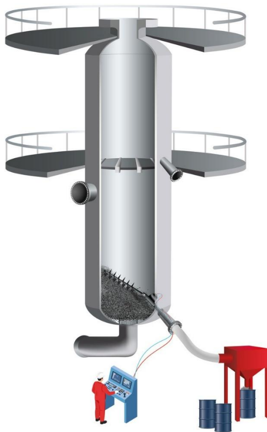
Figure 26: Endless screw excavating the dig-out after gravity dumping
