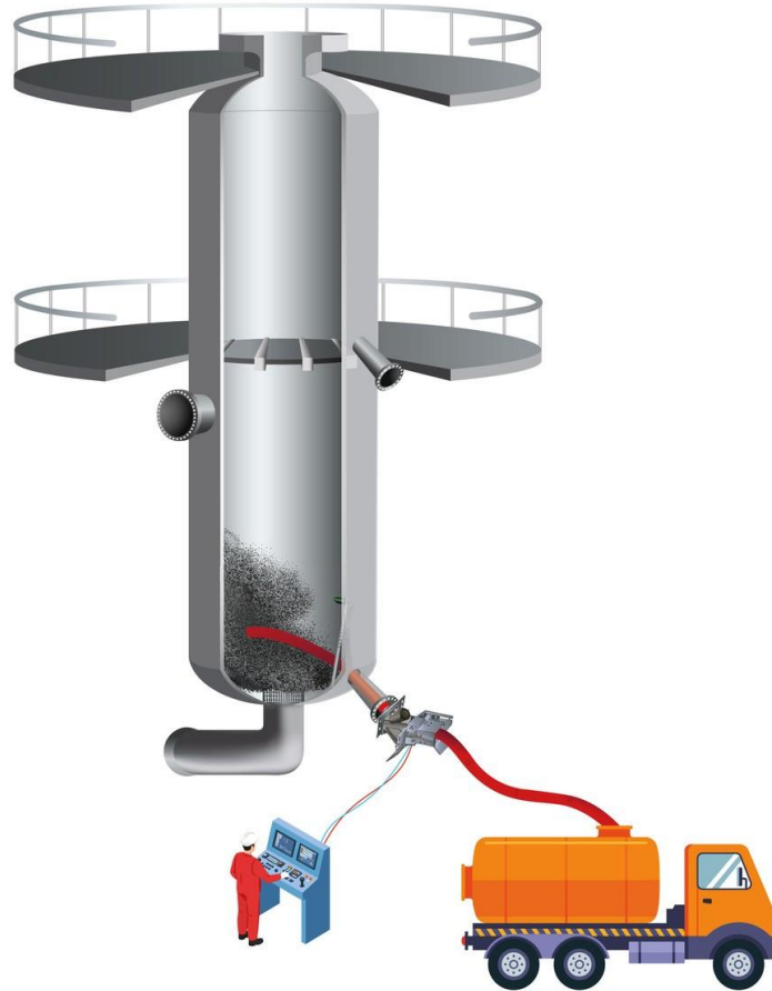
Figure 27: Vacuum hose introduced through the dump pipe
