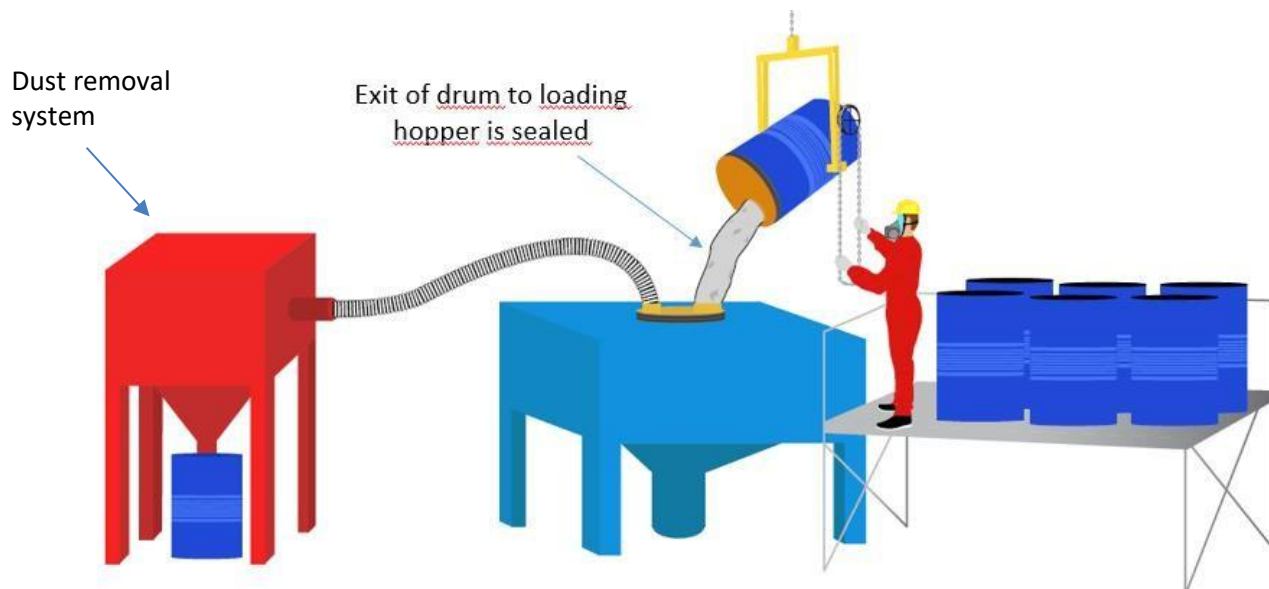
Figure 10: Pre-bagging/filling at ground level where big bag or drum emptying can be better managed and the hopper is lifted by crane.
